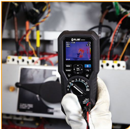
Thermal scan of an electrical panel
