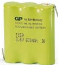
T159 Voltage: 3.6V Capacity: 600mAh Configuration: 60AAM3B1P
