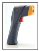
The infrared thermometer Models ST660 , ST662 and ST663 are non-contact infrared temperature measuring instrument . The wide temperature reading from -50~999°C (-58~1830°F) keep users far away from the potential risks.
