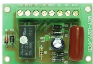
MKT-102 Telephone Ringer Control DPDT Relay Output( 1.25A) Power Source : Phone Line
