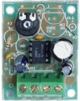
MA-1001 1W Audio Amplifier Power : DC12V
