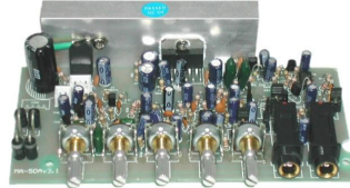
MA-50KT 20W Mini Amplifier Board 2 Microphone & 1 Aux Input Low Impedance Output(4~8Ω) Power Source : DC12V ~ 24V
