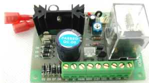
MKT-103 Water Level Alarm Board DPDT Relay Output Load : AC250V / 5A Power Source : DC12V ~ 24V
