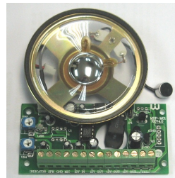
MA-PT Doorphone Talking Amplifier Built-in Call Tone Signal Volume Control For Room & Door Station With 8 Ω / 1.5W Speaker Power : DC12V
