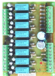
Alarm Control Board MS-4ZAB / 6ZAB / 8ZAB 4 / 6 / 8 Zone Control Board Zone Input : N.C. Contact LED Outputs For Zone Indication 2 Outputs For Buzzer & Strobe Power Source : DC12V (24V) Dimensions : 116 x 78mm
