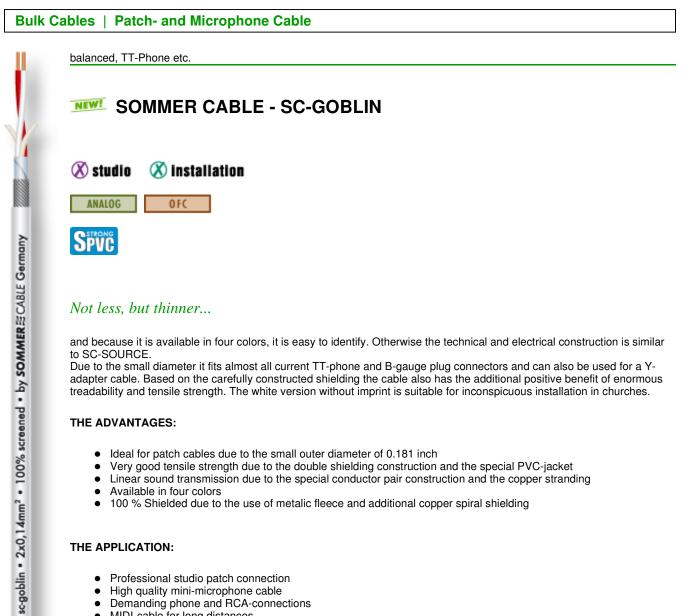
and because it is available in four colors, it is easy to identify. Otherwise the technical and electrical construction is similar to SC-SOURCE.
