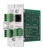
The ZP-001T is a zone paging module designed for use with the M-9000 and functions as interface to connect the M-9000 to an analog PABX, allowing zone paging to be initiated from the PABX. There are two operation modes: ring signal and paging port modes. Broadcast can be initiated regardless of operation mode.
