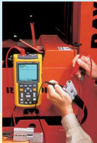
Switch-on and open measure menu to select from 26 scope and meter measurements.
